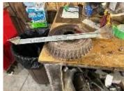
tory 64 Monza brake drum with head dissipatflanges The drum is rusty but hasn't been turned and needs
