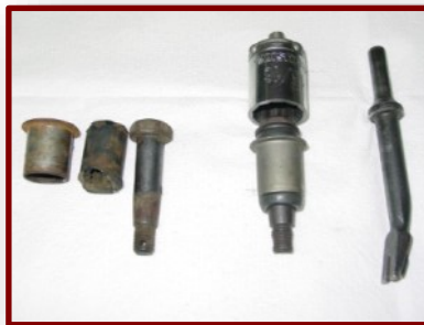
On the left is an old bushing that has been removed. In the center is a new bushing with a home made pusher. On the right is an air hammer tool for removing the sleeve from the center link.
