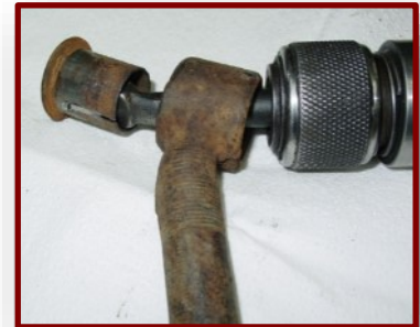
The pressed in sleeve has been removed with the center link still attached to the tie rods
