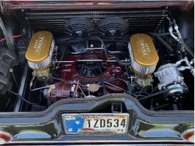
180 hp Yenko Stage II engine build 164 cu. in. bored .060 over 10.00 : 1 compression Isky 280 cam ported heads & headers 4 speed manual transmission
